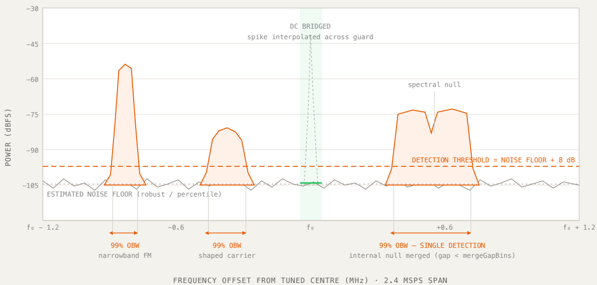
Figure 1. A representative Welch-averaged spectrum frame with the detector's decision structures annotated. Three emitters cross the 8 dB threshold above the robustly estimated noise floor; each is reported with its ITU 99% occupied bandwidth measured in noise-subtracted linear power. At the tuned centre the RTL2832U's permanent DC spike (dashed) has been bridged by linear interpolation across the guard region rather than blanked, so an emitter tuned directly onto centre is not split into two half-width detections. In the wideband emitter at right, an internal spectral null narrower than mergeGapBins is merged rather than fragmenting the emission into two reports.
